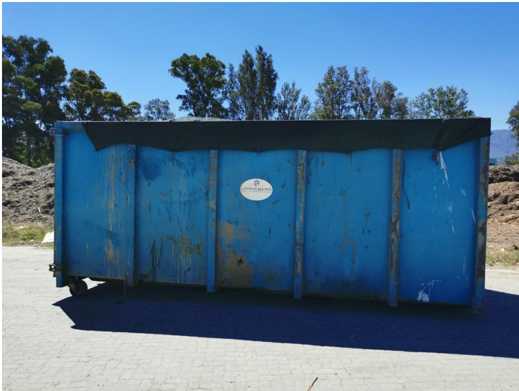
Bent U Channel stiffing ribs, 3mm Mild Steel side cladding
